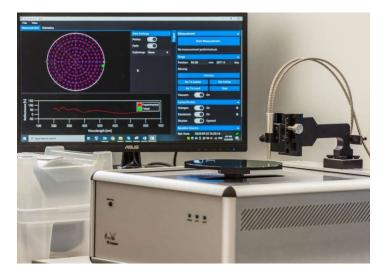
**FR-Scanner** scans the wafers by rotating the wafer and by moving it linearly (Polar Coordinates) with unparalleled speed and accuracy in both radius and angle. This way, accurate reflectance data with high repeatability are recorded, making FR-Scanner the ideal tool for at-line and on-line characterization of coatings on wafers or other substrates at processing facilities.
