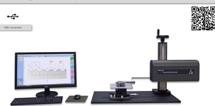
The PGS100 profilometer allows to acquire 2D profiles in an extremely simple and intuitive way, thanks also to its measuring range of 130 mm in length (X) and 50 mm in height (Z).
