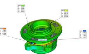
The scanner is available in three basic resolutions: 2x5 MP, 2x9 MP, and 2x20 MP for application that focus on high detail representation. The system can be additionally equipped with a set of exchangeable lenses, allowing a customer to change the scanning volume and adapt to different dimensions or complexity of scanning details.
