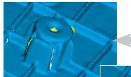
Triangle mesh from a 3D scanner with a resolution of 20 MP (Field of view 480x350 mm)
