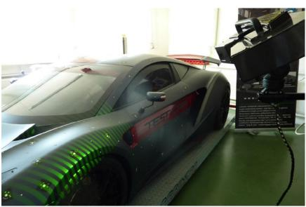
MICRON3D green stereo is a professional, factory-calibrated metrology tool, certified by the manufacturer according to the German VDI / VDE 2634 standard, and its measurement accuracy can be additionally confirmed by a certificate of an independent accredited metrology laboratory.
