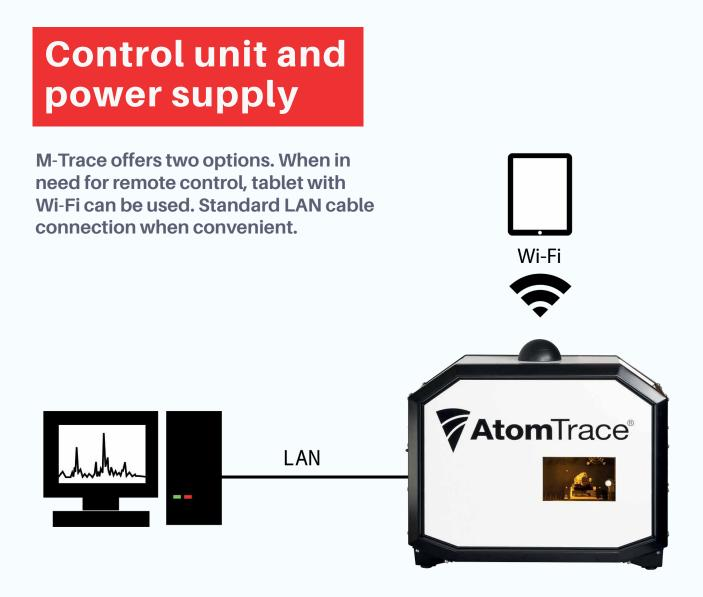
The client-server architecture detaches control and allows remote manipulation with the device via network communication channels Wi-Fi 2.4 GHz, 5.0 GHz, GSM, 3G and LTE. Measured LIBS data are along with initial outputs from analysis saved in real time to local data storage in the device. In the sense of Industry 4.0, the measured LIBS data along with the outputs of the analysis could be exported to remote data storage units on the servers or cloud.
